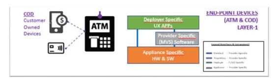
The architecture basic of the ATM end-point device contain Appliance Provider Specific hardware and software shown in orange, can contain Provider Specific Multi-vendor software and other software shown in grey and Deployer Specific User Interface APP shown in green.
