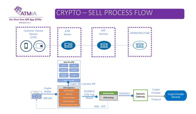
Customer User Interface is not vendor-agnostic and will be ATM deployer FI/IAD specific. The Crypto Currency Provider (provider specific) defines which functionality and technology is supported too, like the Crypto Currency Wallet QRCode.
