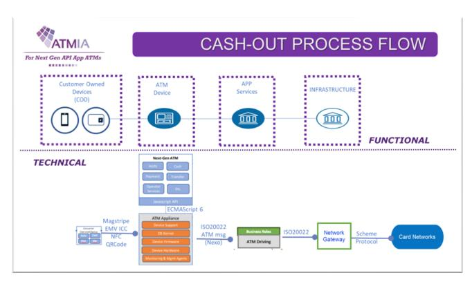
Customer User Interface is not vendor-agnostic and will be ATM deployer FI/IAD specific. The Payment Scheme Specifications defines which functionality and technology is supported too, especially for the endpoints and gateway to the card schemes.
